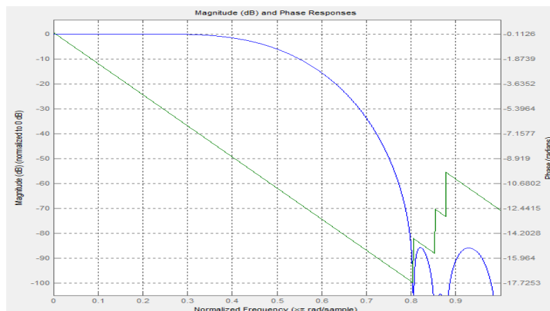
Figure 1: Frequency response of 15 tap desensitized half band filter
